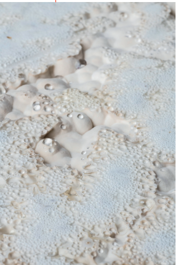
Mycelium-based acoustic panels, produced by Mogu. Alongside, some moments in the process of growing cultures in the molds leading to the finished product.
